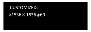
5. EDID modification finished, some PC need to be plugged in and out to enable it.
