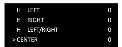
VGA adjustment: adjust VGA input offset.
